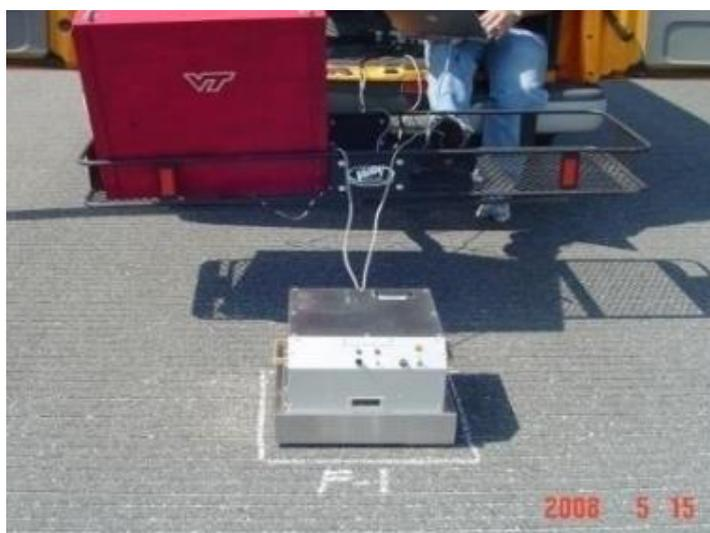
Figure 20 - Circular Track Meter, CTM (Flintsch *et al.*, 2012)
