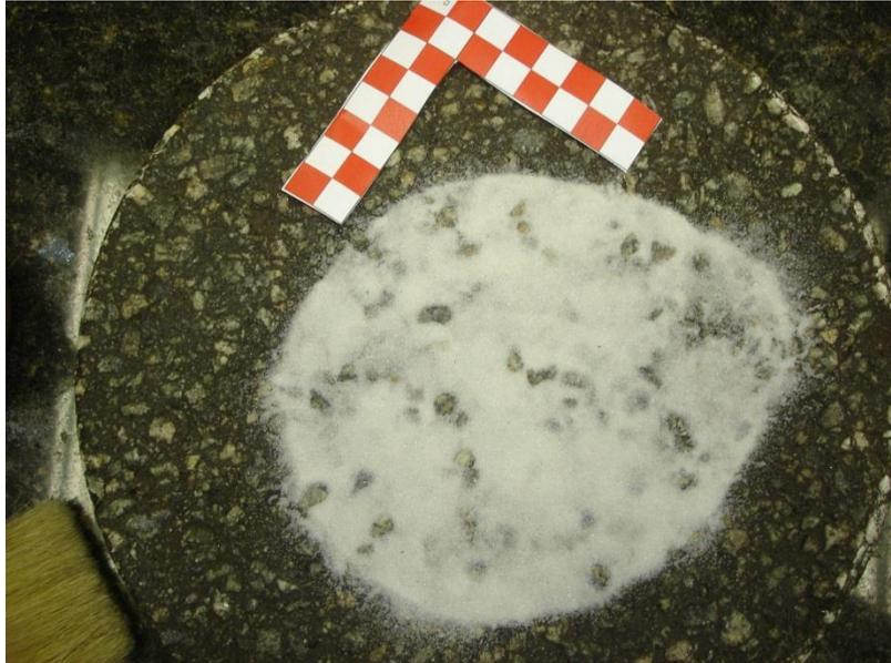
Figure 36 - Sand Patch on a specimen
