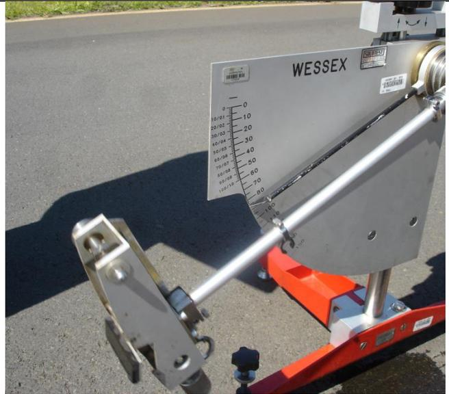
British Pendulum after a measurement. The resulting BPN value is directly read on the scale.
