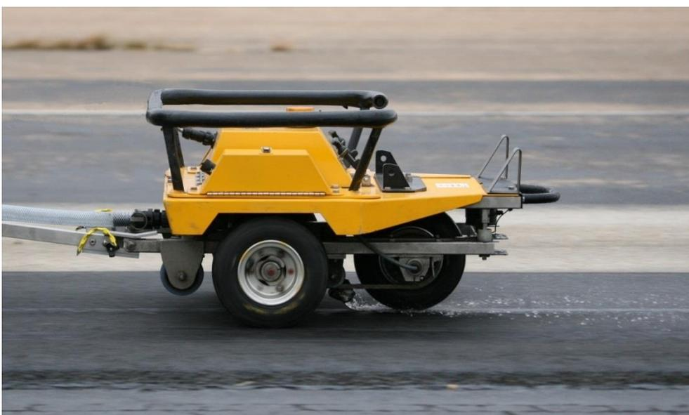
Figure 26 - Locked wheel test with a towed trailer ([www.skid-tester.com](http://www.skid-tester.com))
