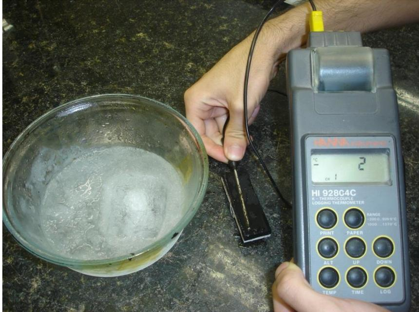
Figure 32 - Rubber slider temperature control, 0°C testing condition
