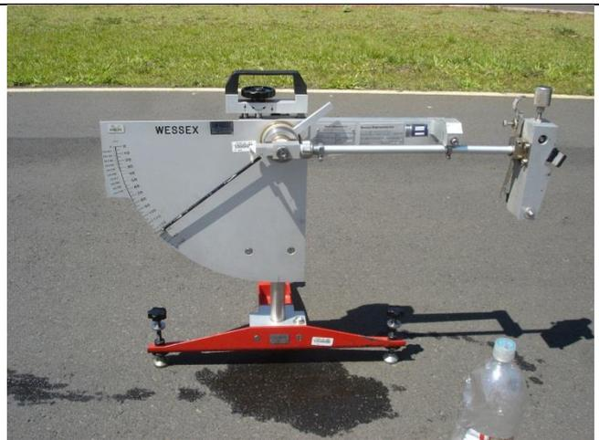
The energy equation for the British Pendulum results in equation eq.38, relating the difference between the initial arm's center of gravity,  $H$ , the highest point reached by the center of gravity after contact,  $h$ , corresponding to the instrument pointer, and the arm weight,  $W$ .
