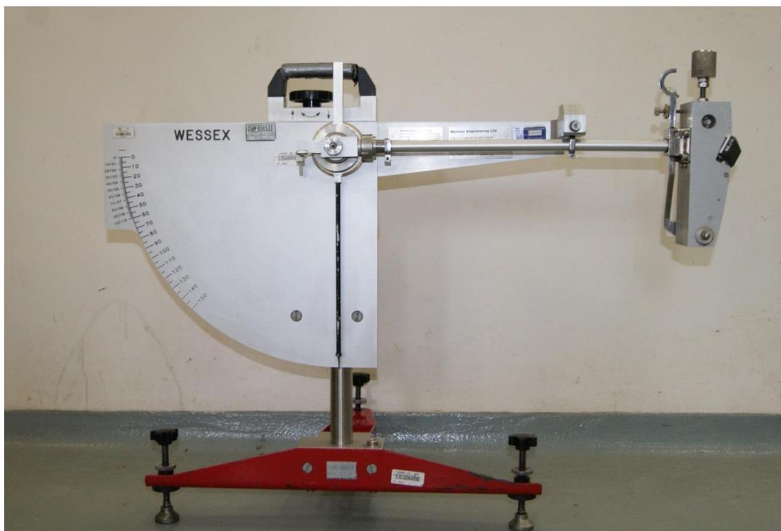
Figure 27 - British Pendulum Tester
